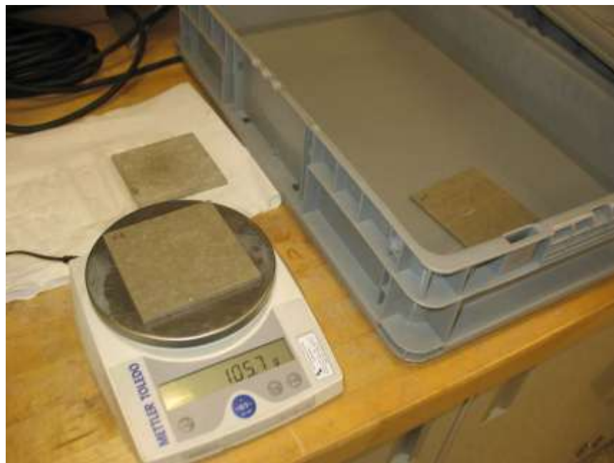
Photo No. 4 Absorption Test Setup
