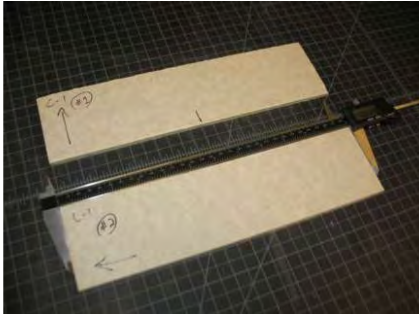
Photo No. 3 Moisture Movement Specimens
