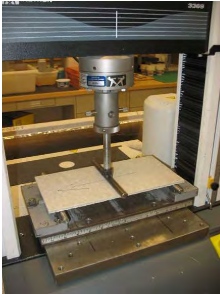
Photo No. 1 Flexural Evaluation Test Setup
